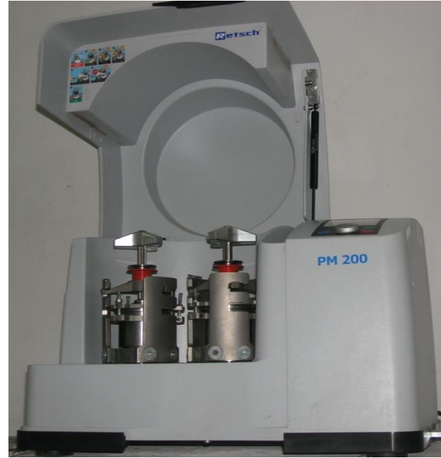
High Energy Ball Mill for synthesis of Nano materials
