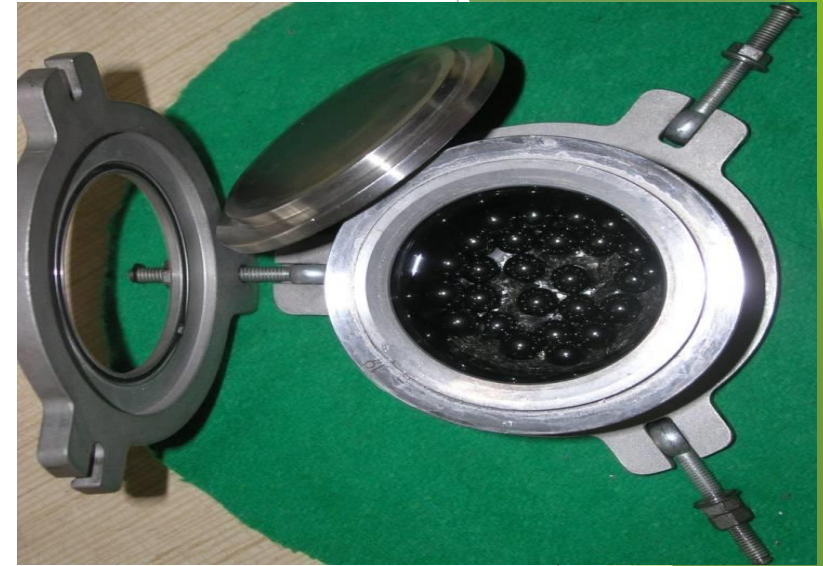
High Energy Ball Mill for synthesis of Nano materials
